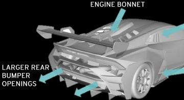
LOWER PRESSURE IN REAR WAKE DUE TO THE SPOILER PRESSURE INCREASE INCREASED ENGINE COMPARTMENT WASHING INLET AREA (In Style Realease rev. 1)
